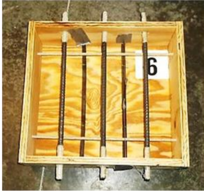
Figure 6 Wood Mold and Steel Reinforcement Configuration
